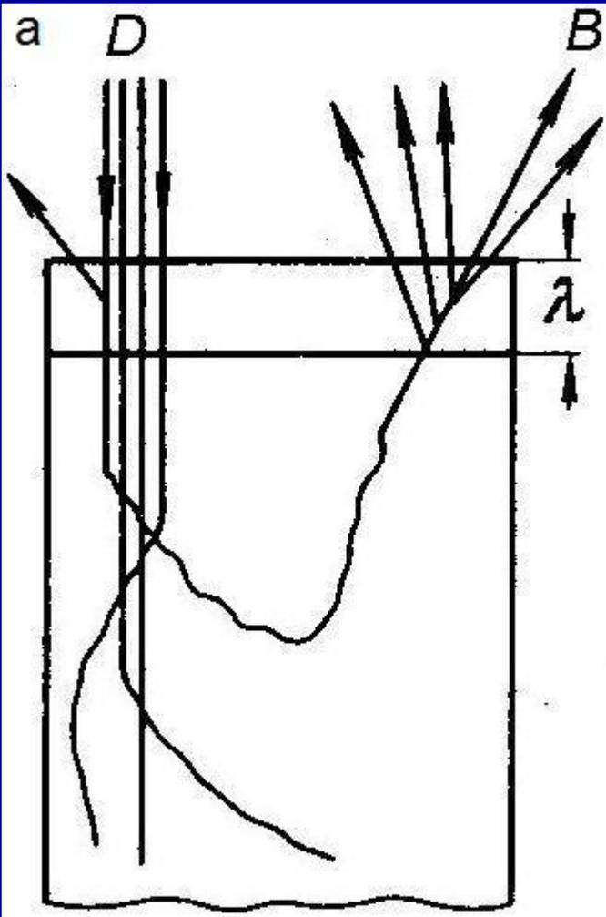
Secondary electrons are produced by backscattered electrons
