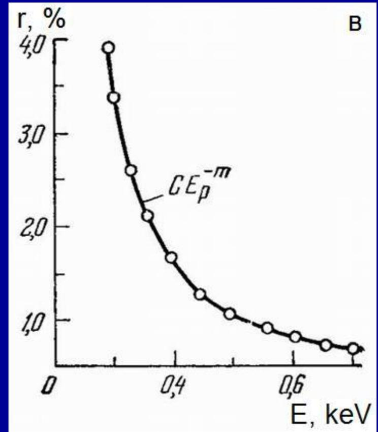
$\sigma$ - secondary emission coefficient
