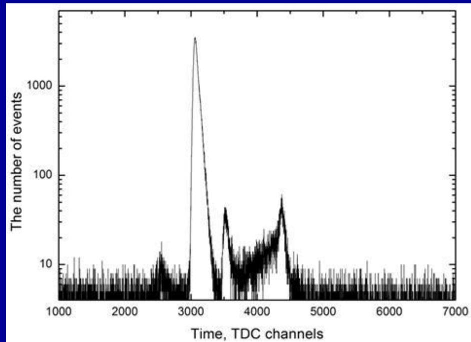
Jitter -  $\sim 4,7$  ns (FWHM); QE $\sim 23\%$  at 400 nm
