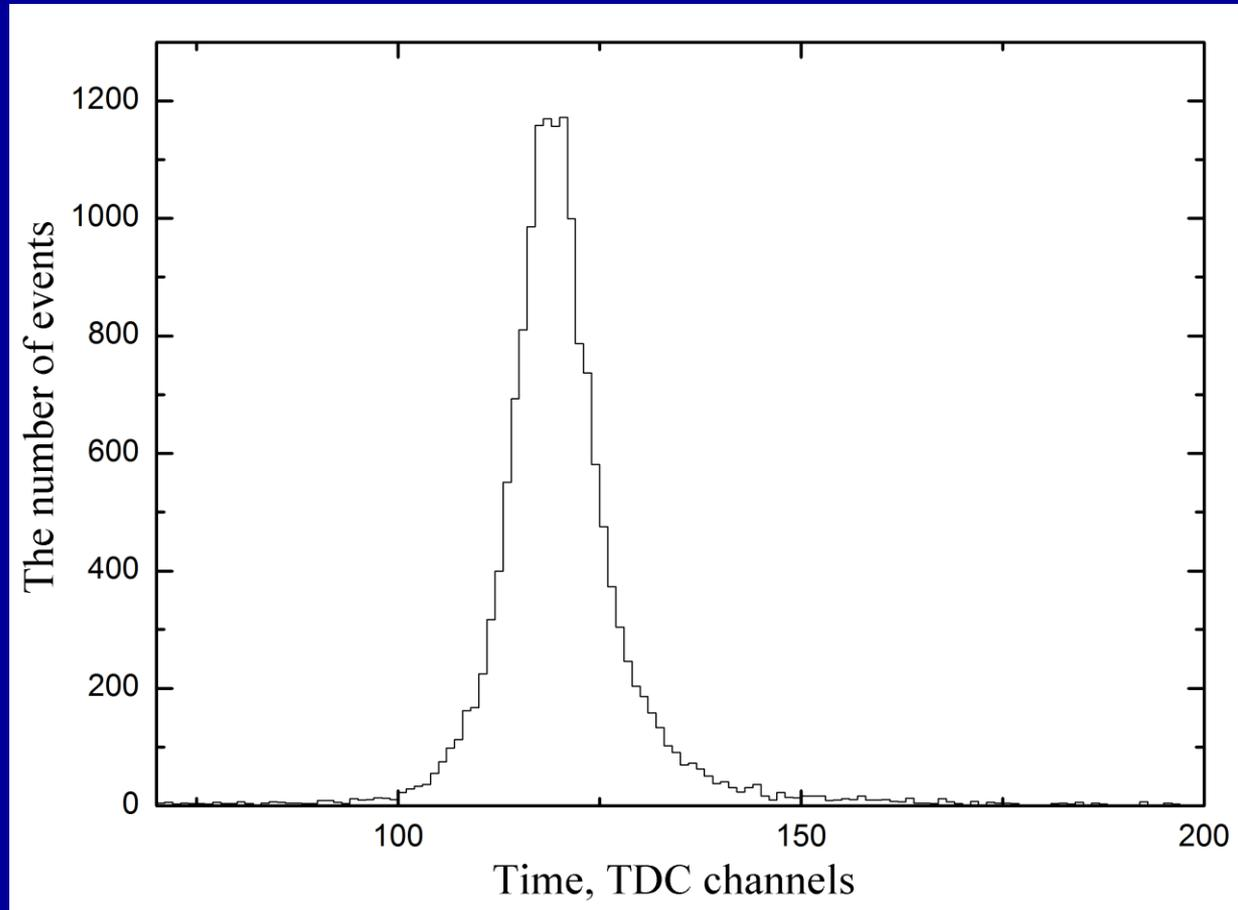
$$\Delta t_{\text{hpd}} \sim 750 \text{ ps (FWHM)}; \quad \Delta t_{\text{LED}} \sim 700 \text{ ps}$$
